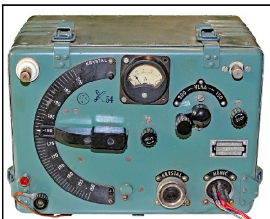
Example of an Eastern Block transmitter, type RS1 6K, with its dial calibrated in 25kHz segments, set to FW 180 = 4.5MHz. (FW 150 to 200 on the dial equalled 3.750 to 5MHz).
